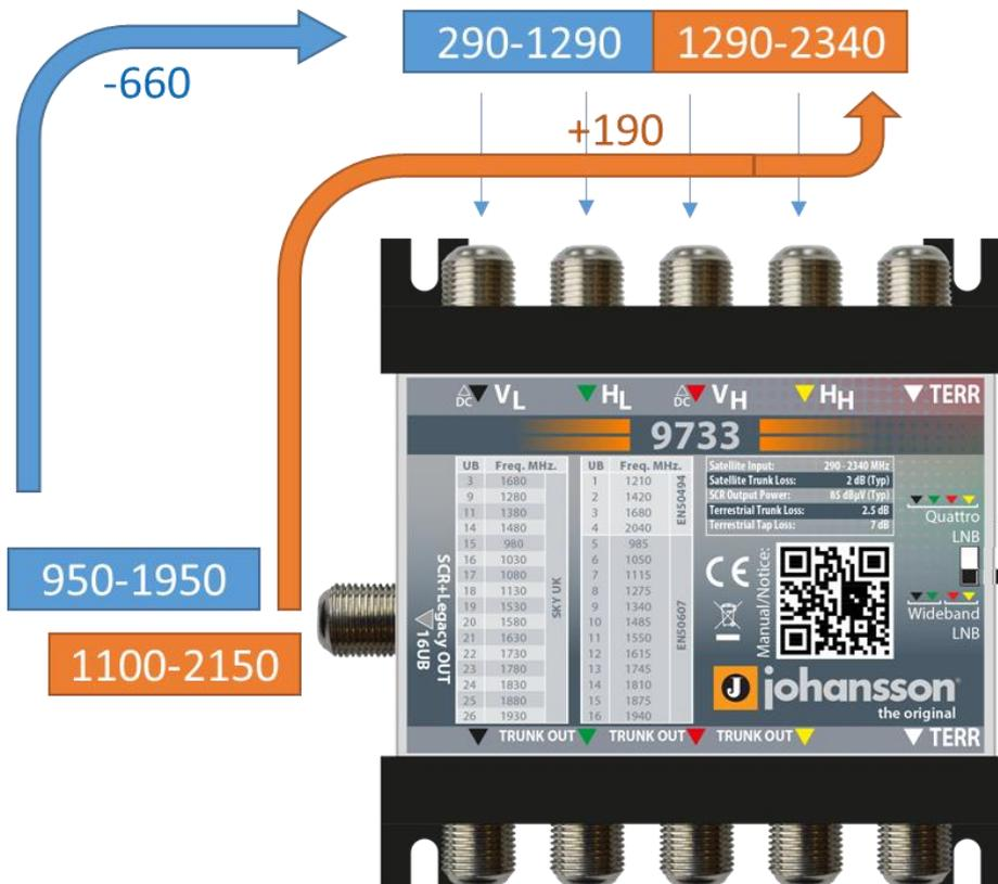
In both the Quattro and Wideband mode, the 9733 / 9734 will allow powering the LNBs on both vertical trunks lines (see chapter 2.3 "DC Power" for more details on how to power the units and the LNB).
